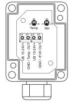
If only the humidity output is used, terminal "UB 15-24V= (Temp)" has to be bridged to "UB 15-24V= (rH/rF)", and terminal temperature output "GND/Temp. OUT 4-20mA" has to be bridged to "GND" of the power supply.
